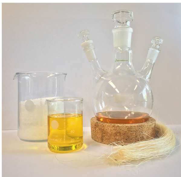
Raw materials used: lactide, vegetable oil and natural fibers as well as one intermediate stage of polymer synthesis in the reaction flask.
