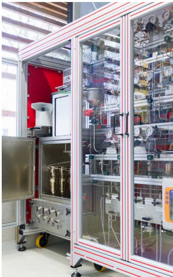
Screening station for testing the synthesis of green ammonia.
