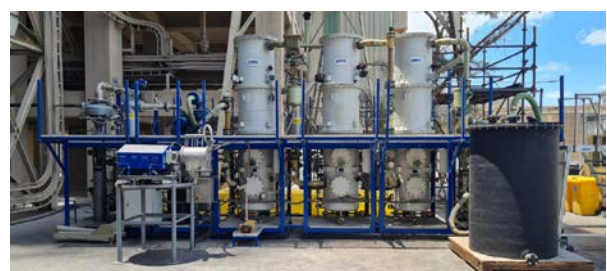
Pilot plant for combined exhaust gas treatment, carbon capture, storage and conversion.
